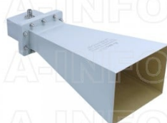
LB-430-10-C-NF Standard Gain Horn Antenna 1.7-2.6GHz 10dB Gain N Type Female
