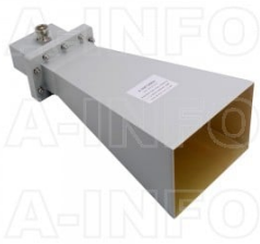
LB-430-10-C-7/16F Standard Gain Horn Antenna 1.7-2.6GHz 10dB Gain 7/16(DIN) Female
